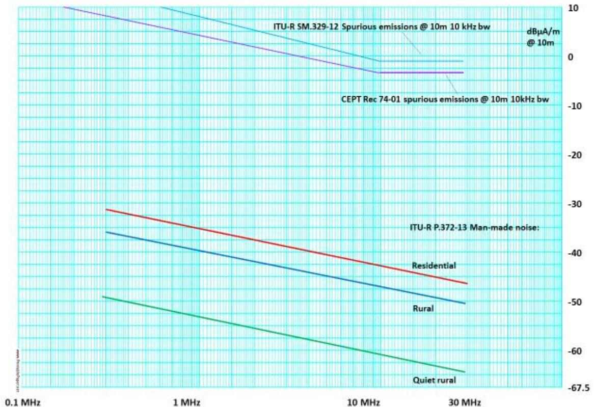
**It is clear that the emissions at 10m distance exceed the median man-made noise figures by 30-45 dB.**
