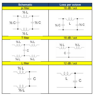
Fig. 8. Types of input filter.
