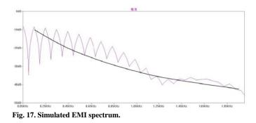
Here, the frequency range of 50Hz to 2kHz is shown as per the standard. Clearly, this design would not pass EN61k testing. The simulator would allow the insertion of low-frequency PFC filters to reduce the amplitude of the higher harmonics as needed but at this power level and the low frequencies involved, the filter would be very large. For this reason, an active PFC circuit should be considered.
