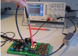
Fig. 12. Using an EMI sniffer probe.
