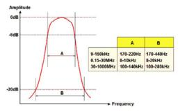
Fig. 6. Bandwidth definitions for EMI measurement.
