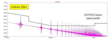
Fig. 18. Simulated spectrum without EMI filter.
